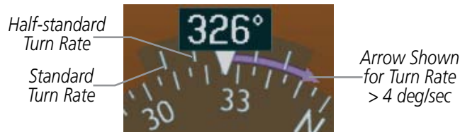
Figure 2-20 Turn Rate Indicator and Trend Vector
